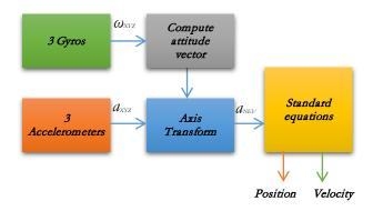
Figure 12. Strapdown INS unit block diagram.
