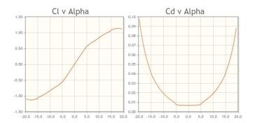
Figure 8. Eppler E838 Hydrofoil characteristics ( $Re = 10^6$ ).
