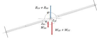
Figure 5. Roll forces balance.
