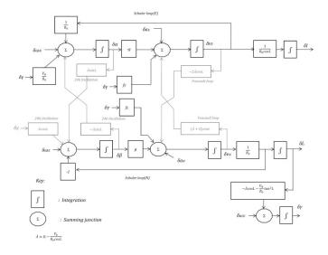
Figure 13. INS long period errors correction block scheme.
