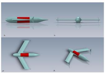
Figure 1. SQUID TUG (Tailless Underwater Glider) view.
