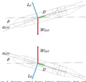
Figure 7. Dynamic vertical forces balance (immersion (top) and emersion (bottom) phases).
