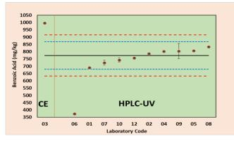
Figure 2. Participant results for MICPT-14-01: Benzoic acid in Mango Juice using capillary electrophoresis and high-performance liquid chromatography with UV detector.
