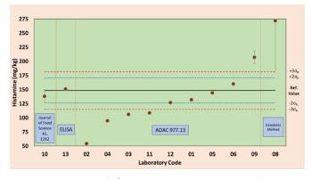
Figure 3. Participant results for MICPT-14-04: Histamine in canned tuna using fluorometer detection with different sample preparation.
