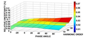
Figure 17. Non Active Power Uncertainty Estimation vs harmonic order and fundamental frequency.
