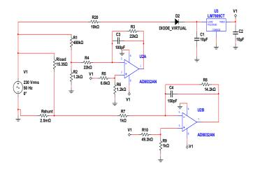
Figure 2. Circuit diagram of the CVCT.
