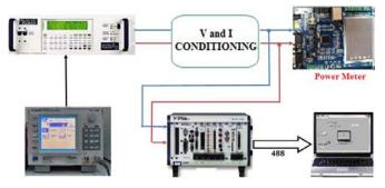
Figure 13. Experimental set-up for dynamic characterization.
