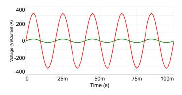
Figure 4. Voltage and current at the input of CVCT.
