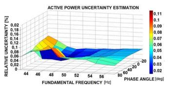
Figure 14. Active Power Uncertainty Estimation vs phase angle and fundamental frequency.
