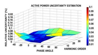
Figure 16. Active Power Uncertainty Estimation vs harmonic order and phase angle.
