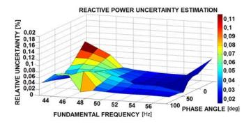
Figure 15. Reactive Power Uncertainty Estimation vs phase angle and fundamental frequency.
