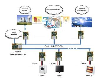
Figure 1. Architecture of the proposed smart metering network.
