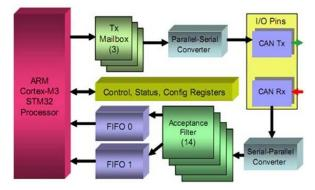
Figure 7. CAN communication device architecture.
