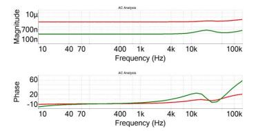
Figure 6. AC analysis of the realized CVCT: magnitudes and phases of the outputs.
