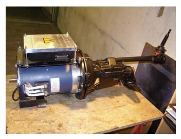
Figure 3. Induction motor with gearbox.
