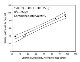
Figure 3. Correlation between results found by Fuel cell and Alcohol oxidase biosensor.
