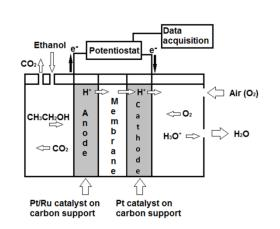
percentages of ethanol were added to the cell, recording the current increase that occurs between two electrodes of the cell,
