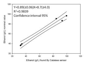
Figure 6. Correlation between nominal values and results found by Catalase biosensor.
