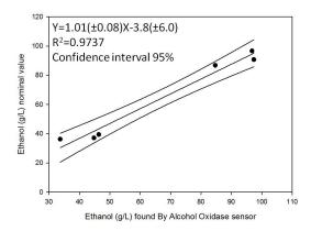
Figure 7. Correlation between nominal values and results found by Alcohol oxidase biosensor.
