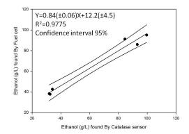
Figure 2. Correlation between results found by Fuel cell and Catalase biosensor.
