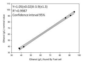
Figure 5. Correlation between nominal values and results found by Fuel cell.
