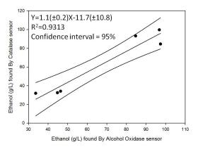
Figure 4. Correlation between results found by Catalase biosensor and Alcohol oxidase biosensor.
