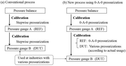
Figure 2. Dissemination process of the pressure standard using pressure gauges: (a) conventional process using stepwise pressurization, (b) new process using 0-A-0 pressurization for the reference pressure gauge.
