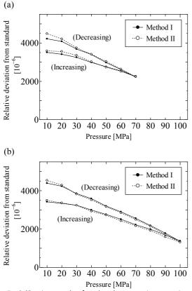
Figure 5. Calibration results for the demonstration experiment with stepwise pressurization for  $p_{max}$  of (a) 70 MPa and (b) 100 MPa.
