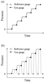
Figure 4. Pressurization procedures for reference and test gauges during calibration. (a) Conventional method, (b) proposed method. For both procedures, the test gauge is calibrated by stepwise pressurization. Timing of the measurements is shown by open circles for the reference gauge, and filled circles for the test gauge.
