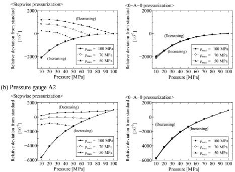
Figure 3. Calibration results for two clamped thin-film pressure sensors with maximum pressures of 50 MPa, 70 MPa, or 100 MPa. (a) Pressure gauge A1, (b) pressure gauge A2. Results for stepwise and 0-A-0 pressurization procedures are compared.
