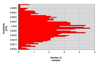
Figure 7. Histogram of the noise-equivalent magnetic field of the 3MH5 SENIS' Teslameter with the low-noise hybrid Hall probe, in the magnetic measurement range 2 T and a frequency range from 0.1 Hz to 10 Hz. The calculated standard deviation is 1.2  $\mu T$  and the six sigma peak-to-peak noise is 7.2  $\mu T$ , which corresponds to the width of the histogram. At DC measurements (integration time 1 s) the teslameter has a peak-to-peak resolution of about 1 ppm of the measurement range.
