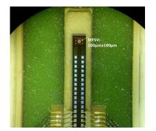
Figure 6. SENIS 3D Hall Probe. Spacial Resolution:100  $\mu$ m x 100  $\mu$ m The probe is packaged in alumina ceramics. Probe dimensions (WxThxL) in mm: 6.0x1.6x14.5.
