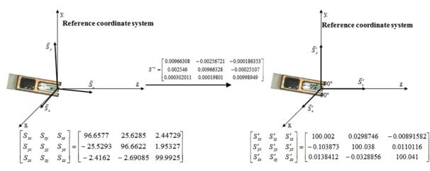
Figure 10. Illustrating the correction of the angular errors of a 3-axis integrated Hall probe [23]. In order to demonstrate the efficiency of the calibration method, the probe was rotated with respect to the z-axis for about 15°. Left: the "raw" sensitivity matrix (before calibration); middle: the inversed "raw" sensitivity matrix; right: the corrected sensitivity matrix, which is an almost identity matrix, with negligible off-diagonal terms. The related angular errors are shown in Table 6.
