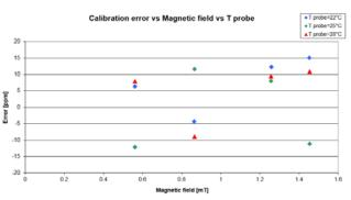
Figure 9. The measurement error of the 3MH5 SENIS' Teslameter in the measurement range 2 T. If the room temperature varies within +/-3 °C around 22 °C, the measurement error is within +/-15 ppm (parts per million) of the measured value.
