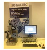
Figure 4. Bomatec AG utilizes the SENIS Magnetic Field Mapping System for quality control of permanent magnets.
