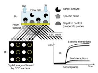
Figure 2. SPRi technology. The receptor is immobilized on the sensor chip gold surface while the ligand is added in solution. From the interaction, a change in the signal is recorded, in label free and real time mode. Parallel analysis on different spots can be performed. The image analysis also visualizes changes on the different spots, providing spatial resolution to the sensorgram changes.
