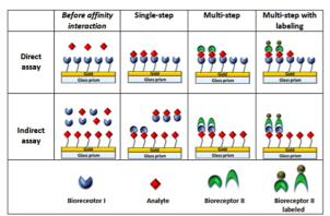
Figure 4. Schematic representation of different strategies for biomolecular recognition, i.e. by direct and indirect detection. Both approaches can be based on single- or multi-step assays, with or without the presence of labels.
