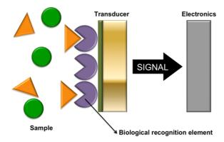
Figure 1. Biosensor scheme: Bio or biomimetic receptors are immobilized on the transduction surface and are responsible of the system selectivity. The binding with the analytes generates an analytical recordable signals whose nature depends on the transduction principle.
