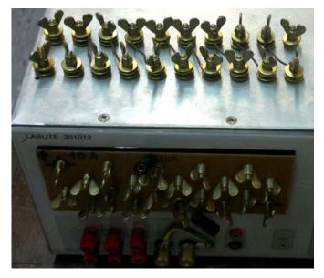
Figure 7. Connection terminals for high-current windings at the upper side of the case.
