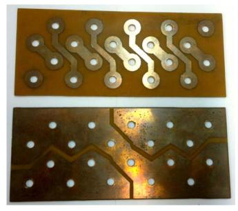
Figure 6. Circuit printed boards used to connect the groups of low-current primary windings. The upper one corresponds to 1 A of nominal current (100 turns), and the lower to 5 A (20 turns).
