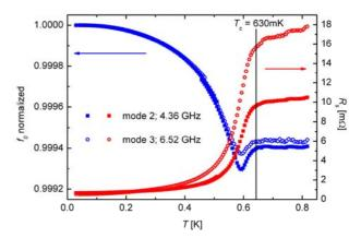
Figure 4. Temperature dependence of stripline resonator frequency  $f_0$  (normalized to the frequency at the lowest temperature) and sample surface resistance  $R_s$  measured on a CeCu<sub>2</sub>Si<sub>2</sub> single crystal sample. Both quantities are shown for two different resonator modes.
