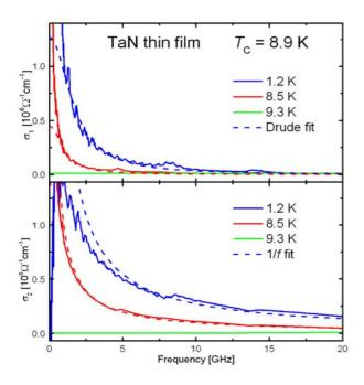
Figure 2. Microwave conductivity spectra of a TaN thin film, measured with a Corbino spectrometer.
