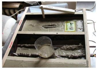
Figure 4. Preparation of concrete specimen with embedded RFID sensor tag.
