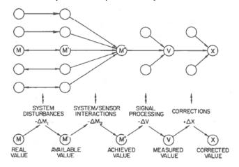
Figure 1. The measurement chain.
