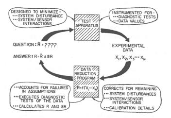
Figure 2. The experimental loop.
