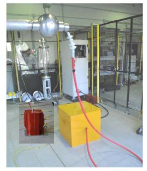
Figure 6. Voltage calibration with the divider inside a metallic grounded box.
