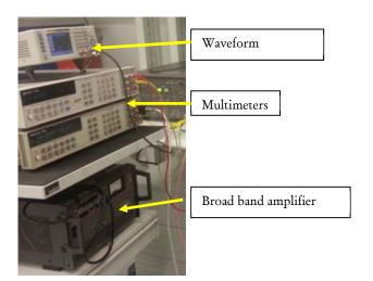
Figure 5. Measurement set-up for the Subsampling configuration.
