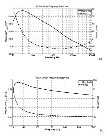
Figure 3. Frequency behaviour of RCD divider between 10 Hz and 90 kHz (a) and zoom between 10 Hz and 300 Hz (b).
