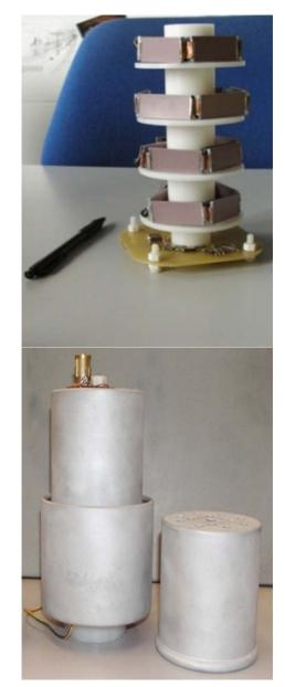
Figure 1. Resistive-capacitive shielded divider during the assembly step.
