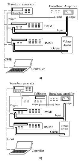
Figure 4. Measurement set-up for sub-sampling digitizing method (a) and for DCV method (b).
