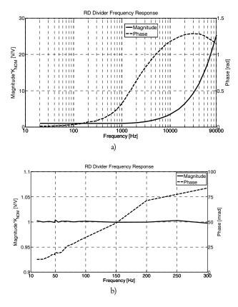
Figure 2. Frequency behaviour of RD divider between 20 Hz and 90 kHz (a) and zoom between 20 Hz and 300 Hz (b).
