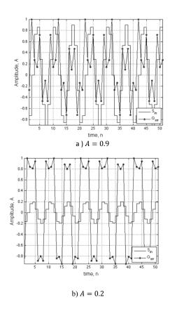
Figure 8. Quantization error of a sinosoid for a 1-bit quantizer.
