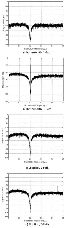
Figure 10 Output spectrums of the FPGA implementation.
