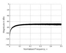
Figure 6. Output spectrum of the Fibonacci LFSR.
