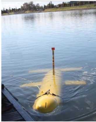
Figure 10. Guanay II AUV in the field test.
