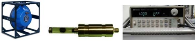
Figure 1. The non-omnidirectional sound pressure generator, Lubell model LL9642T, used as acoustic source (left), the Hydrophone (Björge Naxys Ethernet Hydrophone 02345 used as acoustic receiver (center), and the Signal generator HP33120A (right).
