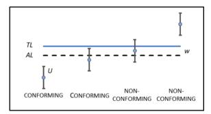
Figure 2. Illustration of the guarded acceptance based on ILAC G8 [1].
