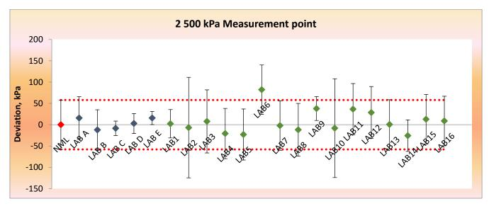
Figure 5. Participant's deviation from the reference values and its corresponding uncertainties at 2500 kPa.
