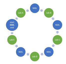
Figure 2. PT 2010 measurement scheme.
