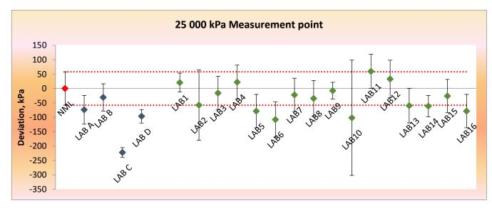
Figure 6. Participant's deviation from the reference values and its corresponding uncertainties at 25 000 kPa.
