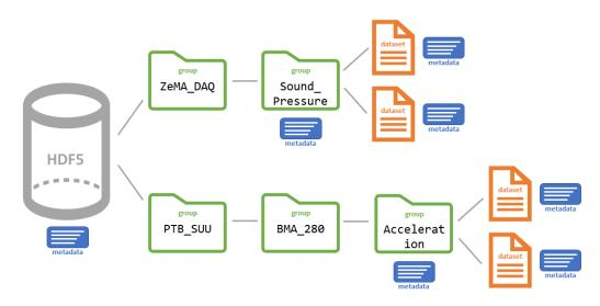
Figure 1. HDF5 file (grey) structure containing groups (green), data sets (orange) and associated metadata (blue).
