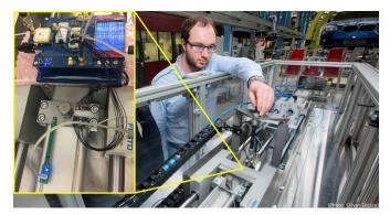
Figure 2. SmartUp Unit (small picture) used together with the ZeMA DAQ for data acquisition of the testbed for an EMC life time test (big picture).
