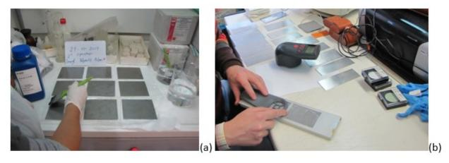
Figure 1. Highlights from laboratory tests during Phase 1: (a) Coating application by brush on uncorroded flat steel specimens and (b) Colour measurements on coated aluminum specimens
