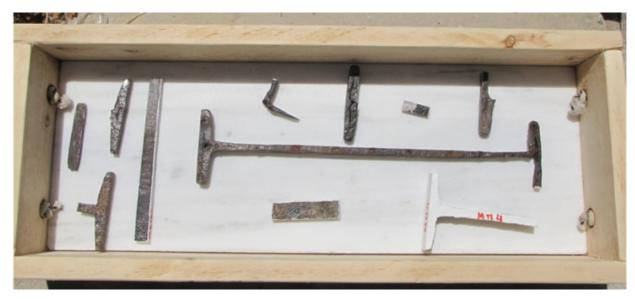
Figure 3. The coated steel joints placed in a marble bottomed open case during field exposure near the monument.
