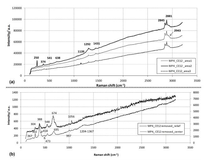
Figure 10. Characteristic Raman vibrations of Poligen CE12 polymer and corrosion products detected after 1 year of field exposure on (a) coated areas of MP4 joint and (b) the same areas after coating removal (brushing with a glass brush)
