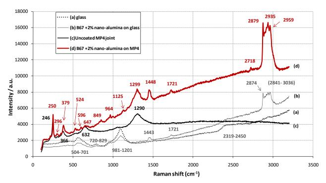
Figure 7. Representative Raman spectra of surfaces coated with Paraloid B67 + 2 % nano- $Al_2O_3$  - The four analysed surfaces correspond to: (a) glass substrate, (b) glass coated with Paraloid B67 + 2 % nano- $Al_2O_3$ , (c) corroded MP4 steel joint and (d) corroded steel joint MP4 coated with Paraloid B67 + 2 % nano- $Al_2O_3$  after 1 year of field exposure.
