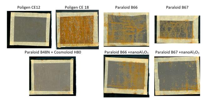
Figure 4. Macroscopic documentation of coated steel specimens after 4 h of exposure in 5 % NaCl salt-spray chamber
