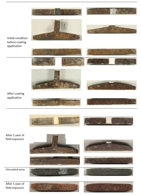
Figure 6. Photographic documentation of joint MP169 (coated and uncoated) at various intervals before and after the coating systems application and after 1 year of field exposure. The uncoated specimen has been significantly more corroded than both coated specimens. The average thickness of the clamp's shaft is 9 mm.
