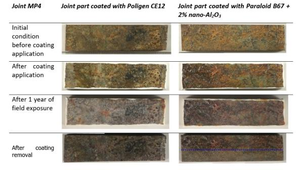
Figure 5. Photographic documentation of joint MP4 before and after the coating systems application and after the coatings removal. Poligen CE12 was removed using a glass fiber brush, while Paraloid B67 based coating was removed using acetone on cotton swabs. The area below the dotted blue line was treated at second stage of Paraloid coating removal with a glass fiber brush. The length of the specimen is about 7.3 cm.
