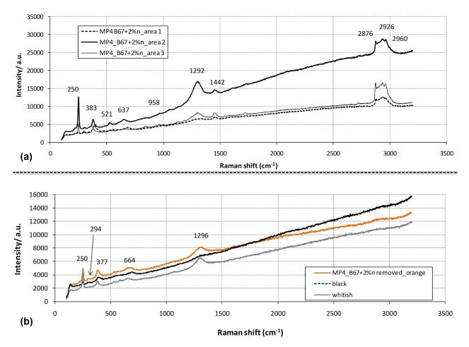
Figure 9. Characteristic Raman vibrations of Paraloid B67 +2 % nano-Al<sub>2</sub>O<sub>3</sub> polymer and corrosion products detected after 1 year of field exposure on (a) coated areas of MP4 joint and (b) the same areas after coating removal (swabbing with acetone and brushing with a glass brush).
