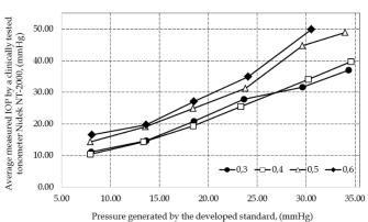
Figure 10. Experimentally found influence of the thickness of the artificial cornea on the non-contact tonometer response as found by the STU.
