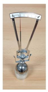
Figure 1. An impression tonometer placed on a precise calibration sphere.
