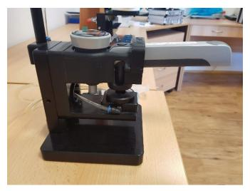
Figure 8. A rebound tonometer on its test bench (detail).
