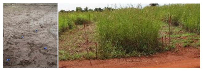
Figure 1. Results from the same demining machine. On the left, test lane used in test site in Germany with dummy Antipersonnel (AP mines), called WORM, 0 cm – 20 cm deep: 98.22 % neutralized. On the right hand side, suspected hazardous area in Angola: 10 AP mines processed and left live intact (of type POMZ and PP-MI-SR).
