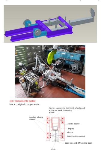
Figure 7. Scheme of Disarmadillo: red parts, frame, wheels, tracks and band brakes are added to the original powertiller (black).
