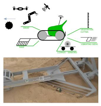
Figure 5. Disarmadillo tools (*top image*) and a picture of the *rake*, tested in Jordan with dummy mines (*bottom image*).
