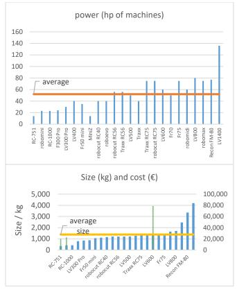
Figure 10. Power, size and cost of remotely controlled agricultural multi platforms currently on the market. In the last graph green bars indicate cost.
