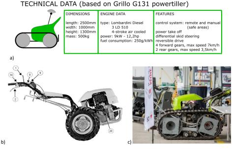
Figure 6. a) Technical data of Disarmadillo machine based on G131 powertiller produced by Grillo. b) The original powertiller and c) Disarmadillo as it was exhibited at the 7<sup>th</sup> Mine Action technology Workshop in Basel in 2019.
