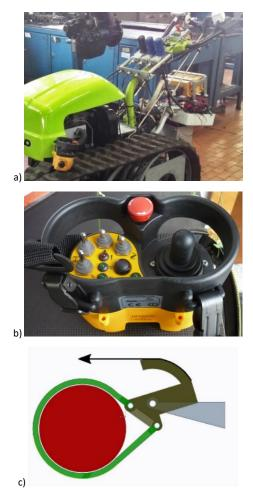
Figure 8. Particular of the control unit: a) linear motors actuating brakes and the clutch, b) transmitter and c) 3D model of band brakes leverage.
