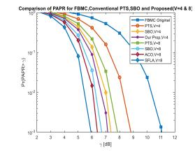
Figure 4. Comparison of PAPR for V = 4 and V = 8 using different methods.
