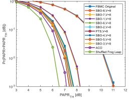
Figure 3. Comparison of PAPR with respect to threshold values.
