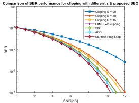
Figure 5. Comparison of BER with respect to SNR.
