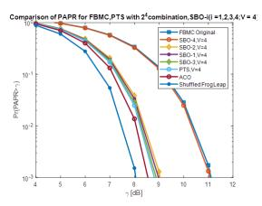
Figure 2. Comparison of PAPR for different techniques.
