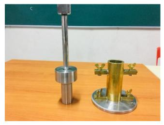
Figure 2. Mini compaction test apparatus.
