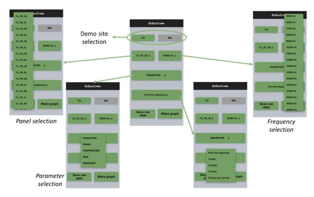
Figure 5. Mobile application for monitoring: selection of demo site, panel and electrode array, measurement frequency and parameters of interest.
