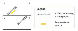
Figure 1. First concrete panel prototype: configuration scheme.
