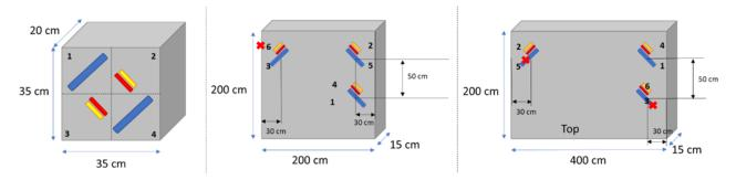
Figure 8. Concrete panels exposed to the demo site in León (Spain): no. 2 panels of 35 × 35 × 20cm³ (left), no. 1 panel of 200 × 200 × 15 cm³ (centre) and no. 1 panel of 200 × 400 × 15 cm³ (right). Legend: 4-electrode arrays with 4-cm spacing are reported in blue, 4-electrode arrays with 1-cm spacing are reported in red, temperature sensors are reported in yellow.
