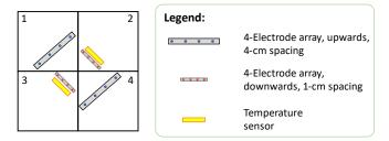
Figure 2. Second concrete panel prototype: configuration scheme.
