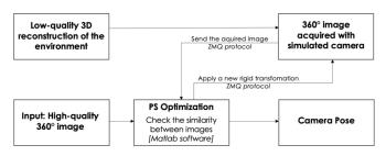
Figure 1. Schematic diagram of the camera pose detection algorithm.
