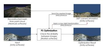
Figure 4. Example of the camera pose detection algorithm flow for the mine
