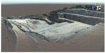
(c) Point cloud obtained projecting the pixels of the  $360^{\circ}$  image on the raw 3D mesh (Unity Software).
