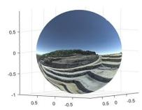
(a) 360° image placed on the surface of a unitary sphere (Matlab Software).
