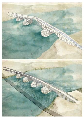
Figure 10. Illustration of the two main phases: the Roman bridge (top); the bridge nowadays showing the foundation *platea* (bottom).
