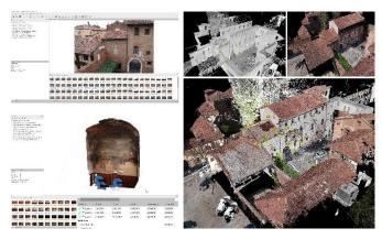
Figure 6. The integrated laser scanner and UAV survey made it possible to fully acquire the internal and external surfaces of the chapel.
