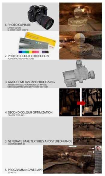
Figure 6. Synthesis of methodological workflow.
