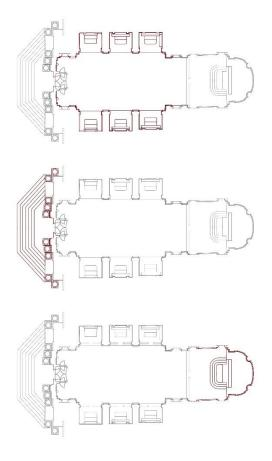
Figure 2. Graphic representation of the three construction phases of the church of Santi Anastasio e Vincenzo in Rome.
