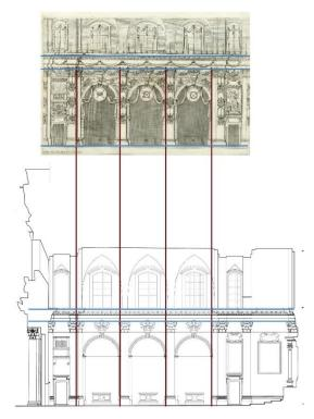
Figure 3. Analysis of the scale and deformation in the engraving of the nave in relation to the survey.
