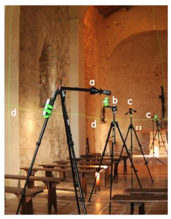
Figure 5. A sample setup:  $\mathbf{a}$  - the 360 camera; oriented horizontally,  $\mathbf{b}$  - a 3 axes laser level,  $\mathbf{c}$  - tripods on which acoustic devices will be mounted,  $\mathbf{d}$  - intersection of laser beams on the interior's enveloppe. (St Pancrace's Chapel, Pyloubier).
