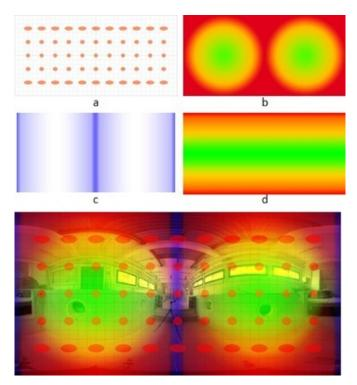
Figure 3. Synthetic image illustrating quality variance of an equirectangular projection composed of: Tissot's indicatrix (a), stitching artifact (b), gradient of equirectangular distortion (c) and gradient of double-fisheye distortion.
