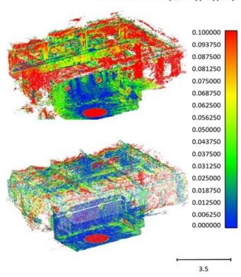
Figure 12. Qualitative comparison tests conducted inside the "fake chapel" (see section 2.1): result of Cloud2Cloud (C2C) distance between laser scanner reference and (top) point cloud generated from a 12k panorama without pyramidal protocol and (bottom) compared to a pointcloud generated from the 5.7K panoramas with pyramidal sequence.
