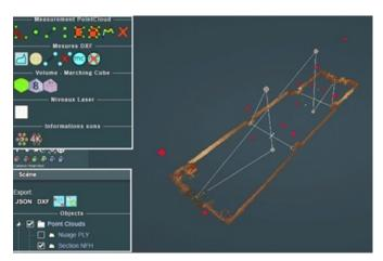
Figure 10. The polyline that corresponds to the scaling protocol (DXF outputted by the Leica Disto, twelve control points), represented inside the *Potree* point cloud renderer. Here only a sub-coud correspoding to the horizontal laser beam is shown.
