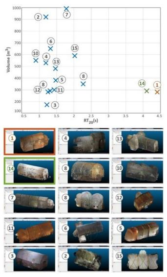
Figure 17. Top: Comparative analysis of data indicators (reverberation time vs. volume) across the collection (top): two items (n° 1 and 14) in the collection stand out significantly due to their high reverberation time and small volume. Bottom: The corresponding point clouds are bordered in colour in the bottom graphics: n° 1, red - N.D de Bethléem (Bras), n° 14, green - Saint-Roch chapel (Les Mées).
