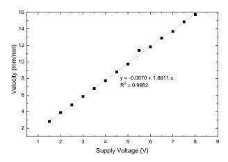
Figure 3. Relationship between the supply voltage to the DC servo motor and the resulting dipping rate.
