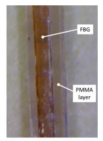
Figure 1. FBG Ethanol sensor with PMMA sensing layer.
