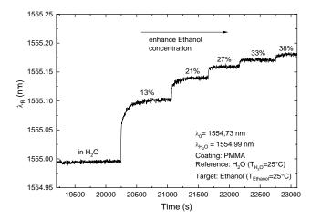
Figure 8. Response of the FBG Ethanol sensor at progressive Ethanol concentrations.
