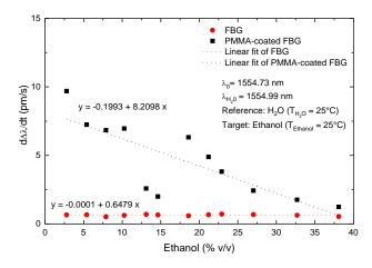
Figure 11. Sensitivity vs. Ethanol concentration for FBG and for PMMA-coated one.
