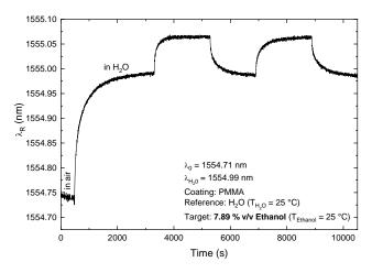
Figure 6. Different response of the FBG Ethanol sensor in air, into distilled water and exposed at a fixed Ethanol concentration (7.89 % v/v).
