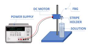
Figure 2. Block diagram of the deposition setup.
