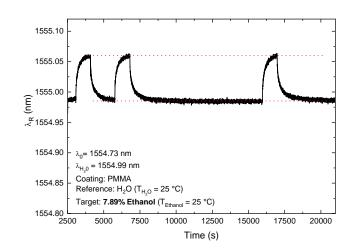
Figure 9. Repeatability of the FBG Ethanol sensor exposed at a fixed Ethanol concentration of 7.89 % v/v.
