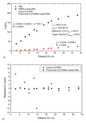
Figure 10. a) comparison between the calibration curves of the FBG and the PMMA-coated one and b) residual analysis of the fittings.
