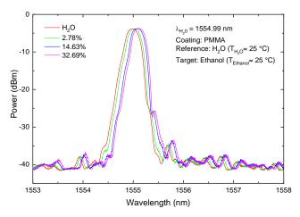
Figure 5. Power spectra of the FBG Ethanol sensor for different concentrations of Ethanol in pure water.
