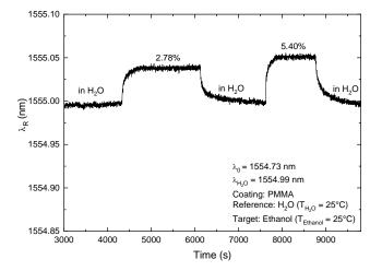
Figure 7. Wavelength shifts after exposition of the FBG Ethanol sensor to different concentrations of Ethanol.
