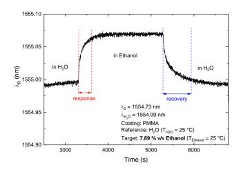
Figure 12. Response and the recovery time of the FBG Ethanol sensor exposed to a fixed Ethanol concentration (7.89 % v/v).
