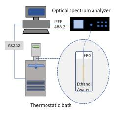
Figure 4. Block diagram of the measurement setup.
