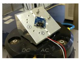
Figure 2: The calibration set-up: the MEMS fixed to the inclined plane on the vibrating table.
