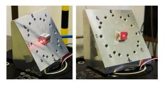
Figure 5: The laser beam hitting the aluminum triangular-based parallelepiped located at the MEMS position.
