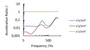
Figure 9: Normalized accelerations along x'-, y'- and z'- axis at 75° of tilt angle.
