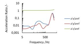
Figure 6: Normalized accelerations along x'-, y'- and z'- axis at 15° of tilt angle.
