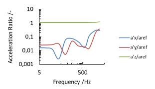
Figure 8: Normalized accelerations along x'-, y'- and z'- axis at 55° of tilt angle.
