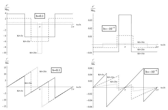
Fig. 3. Velocity and excess density in the standing wave in a resonator filled with chemically reacting gas after formation of the saw-tooth wave, for different values of  $K\theta$  and b.
