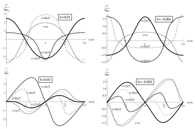
Fig. 1. Velocity and excess density in the standing wave in a resonator filled with chemically reacting gas before formation of the saw-tooth wave, at different fractions of period.
