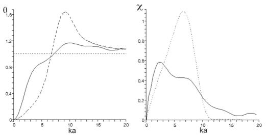
Fig. 4. Impedance of high directivity sound source for  $\alpha_{13}$ : - - - without phase correction, — with phase correction.
