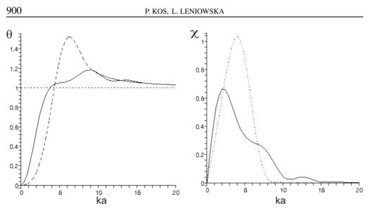
Fig. 3. Impedance of high directivity sound source for  $\alpha_{12}$ : - - - without phase correction, — with phase correction.
