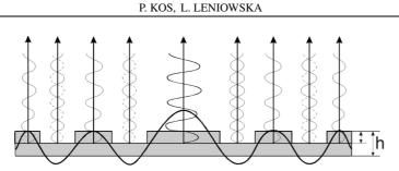
Fig. 1. Explanation of the phenomenon "turning back" the vibration velocity phase on the piston surface.
