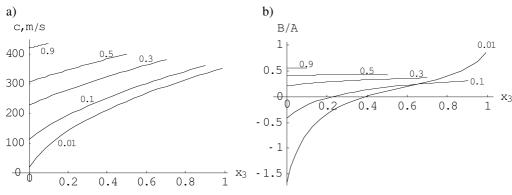
Fig. 2. The small-signal sound velocity c (a) and the parameter of nonlinearity B/A (b) of the ternary mixture consisting of water, its vapor and dry air with separate volumes occupied by air and vapor. The mass concentration of the vapor  $x_2$  has the values 0.01, 0.1, 0.3, 0.5, 0.9 from the lowest to the upper curve in every set. The horizontal axis presents the mass concentration of air  $x_3$ .
