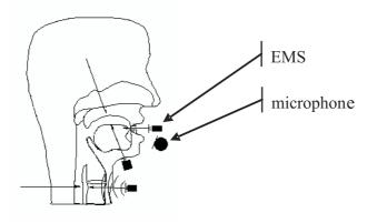
Fig. 3. Sensors' configuration in relation to a patient's head.
