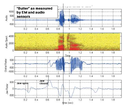
Fig. 4. Example of signals from glottal and jaw sensor.
