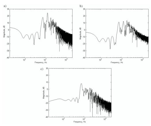
Fig. 3. Filters magnitudes, a) for recording studio-played loudly, b) for anechoic chamber-played loudly, c) for recording studio-played softly.
