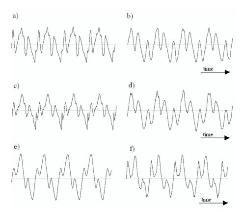
Fig. 4. Time waveforms of the original and simulated sounds: a) original and b) simulated sound for recording studio – played loudly, c) original and d) simulated sound for anechoic chamber – played loudly, e) original and f) simulated sound for recording studio – played softly.
