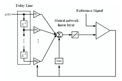
Fig. 2. Block diagram of an adaptive filter.
