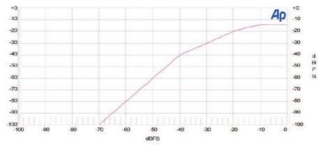
Fig. 4. Static characteristics of the dynamic range controller.
