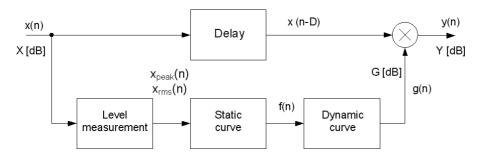
Fig. 1. Block diagram of typical DRC system.
