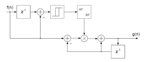
Fig. 3. Block diagram of gain smoothing implementation.
