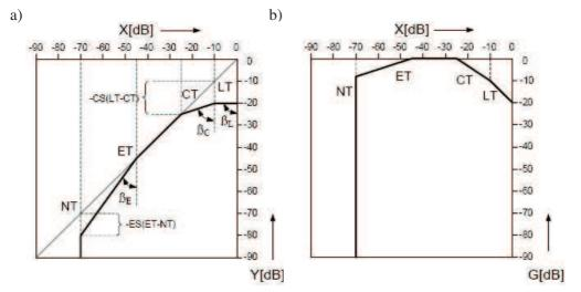
Fig. 2. Static characteristics of the dynamic range controller.
