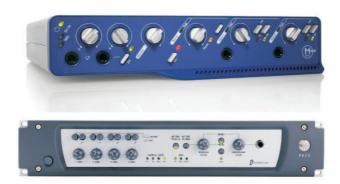
Fig. 1. Multichannel interfaces which enable mixing surround in Pro Tools LE.
