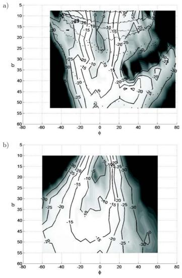
Fig. 6. Comparison between bistatic scattering strengths measured at sea a) and simulated b). From Canepa  $et\ al.\ [13].$
