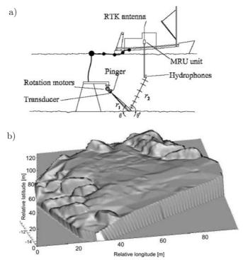
Fig. 5. a) general bistatic set-up used in the NURC experiments [13], b) measurements show the real seabed is not exactly flat, affecting the calculation of scattering strengths.
