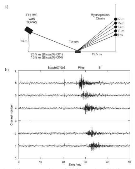
Fig. 7. a) typical bistatic setup used during the SITAR sea trials; the TOPAS-120 transmitter is mounted on the research ROV PLUMS, b) typical signals recorded on the hydrophone chain.
