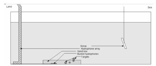
Fig. 4. Full-scale targets are placed in a sand box 10 m (L)  $\times$  5 m (W)  $\times$  0.3 m (D), in the middle of a test basin 80 m (L)  $\times$  10 m (W)  $\times$  8 m (D) later flooded with sea water. The sonar can be tilted to image the targets in the sandbox at different angles of incidence. The hydrophones in the array at the end of the tank allow access to different angles of scattering. Adapted from Zakharia [35].
