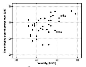
Fig. 6. The effective sound power level  $\widetilde{L}_{WA}$  of heavy vehicles versus vehicle speed V on conventional asphalt.
