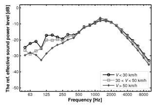
Fig. 3. The referenced level of the effective sound power on conventional asphalt (2000, Pavement A).
