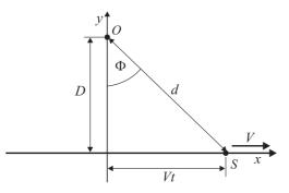
Fig. 7. The source - receiver geometry in the vertical plane.
