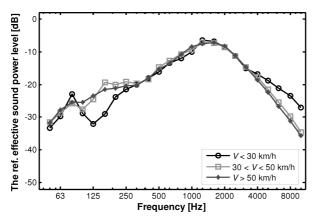
Fig. 5. The referenced level of the effective sound power on porous pavement after three years of use (2003, Pavement A).
