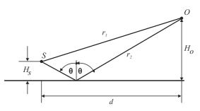
Fig. 8. The source - receiver geometry in the horizontal plane.
