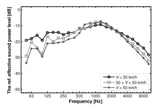
Fig. 4. The referenced level of the effective sound power on new porous pavement (2000, Pavement A).
