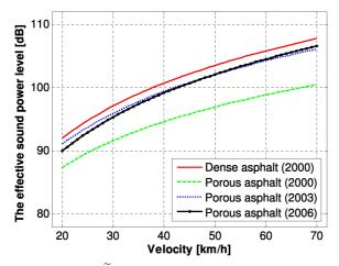
Fig. 1. The effective sound power level  $\widetilde{L}_{WA}$  versus vehicle speed V on conventional asphalt, new porous asphalt and porous asphalt after three and six years of use (Pavement A).
