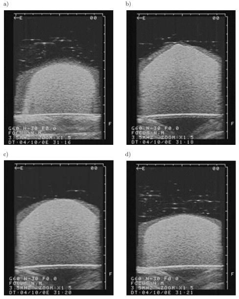
Fig. 7. Examples of US images of transverse cross-sections of the CIRS Model 059 phantom for the following distances of the linear probe axis from the edge of the tank (where inclusions expected): a) 2 cm, b) 5.5 cm, c) 7.5 cm, d) 11 cm.
