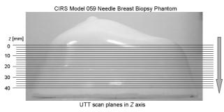
Fig. 3. Way of UTT measurements of individual longitudinal cross-sections of the phantom.
