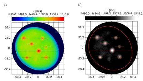
Fig. 10. UTT image of distribution of local values of ultrasound velocity for the CIRS Model 059 phantom longitudinal cross-section for the height of z = 20 mm, with contours of the shape of the cross-section and inclusion edges rendered from a CT image (Fig. 8b): a) rainbow colours image, b) greyscale image with boosted contrast ( $50 \rightarrow 80\%$ ) and reduced brightness ( $50 \rightarrow 32\%$ ).
