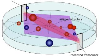
Fig. 13. Exemplary representation of the location of inclusions in the examined structure for the measurement space whose height is equal to the height of the elementary ultrasonic transducers of a ring probe (red inclusions are located in the horizontal plane of the transducer's axis).
