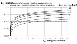
Fig. 12. Calculations of the difference of ultrasound velocity projection values for a breast calculation model with a lesion and without any lesion, depending on the lesion diameter, with the parameter  $\Delta c = 1, 2, 5, 10, 15, 20$  m/s.
