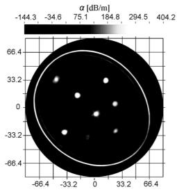
Fig. 14. UTT image of the distribution of local values of the ultrasound attenuation coefficient for the CIRS Model 059 phantom longitudinal cross-section for the height of z = 20 mm, with boosted contrast (50  $\rightarrow$  90%) and reduced brightness (50  $\rightarrow$  43%).
