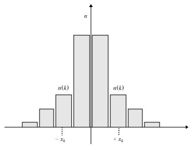
Fig. 2. Space distribution of vehicles in the queue, where n(k) denotes the number of vehicles stopping during the time interval, T, at distance,  $+x_k$  and,  $-x_k$ .
