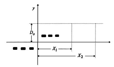
Fig. 4. Microphone location during the simultaneous measurement of the equivalent continuous sound levels,  $L_{AeqT}(X_1)$  and  $L_{AeqT}(X_2)$ .
