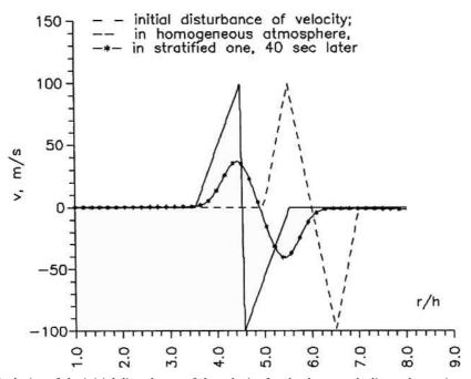
Fig. 1. Evolution of the initial disturbance of the velocity for the downwards directed wave in a stratified and a homogeneous gas.
