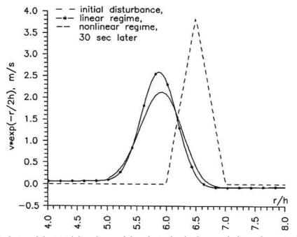
Fig. 2. Evolution of the initial disturbance of the velocity for the downwards directed wave in the linear and weak nonlinear regimes.
