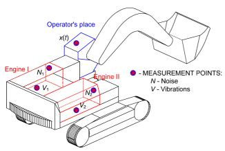
Fig. 3. Distribution of measuring points in a two-motor machine (using the example of a hydraulic excavator).
