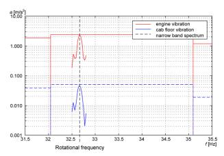
Fig. 8. Example of the vibration accelerations analysis for the signal component of the rotational frequency.
