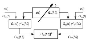
Fig. 6. Schematic presentation of the algorithm for determination of the coherence function with the intermediate signal (reference).
