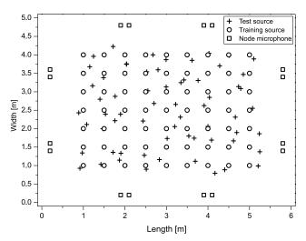
Fig. 2. Acoustic source and node microphone layout.
