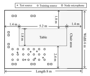
Fig. 9. Layout of node microphones and source positions used for training and testing in real-world experiments.
