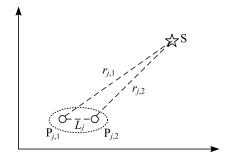
Fig. 1. Acoustic source and node microphone positions.
