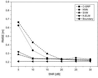
Fig. 4. RMSE of different methods for different SNRs with  $T_{60} = 0.3 \mbox{ s and } M = 630.$
