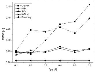
Fig. 5. RMSE of different methods for different  $T_{60}{\rm s}$  with SNR = 15 dB and M = 315.
