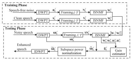
Fig. 4. Block diagram of the proposed speech enhancement system.
