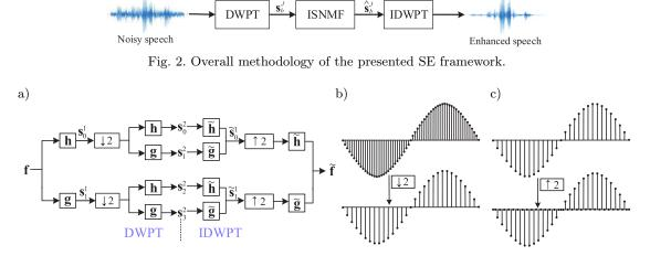
Fig. 3. (a) Flowchart of the two-level decomposition DWPT and IDWT. Here **h** and **g** denote the frequency responses of the low and high pass decomposition filters, respectively. (b) The operation of downsampling. (c) The operation of upsampling. The down arrows represent decimation by 2.
