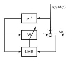
Fig. 2. Prediction-based noise compensation.
