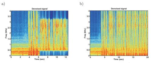
Fig. 12. Spectrograms demonstrating speech enhancement for the first system (system starts at the sample 50000) a) with the additional band-pass filtering; b) without the band-pass filtering.
