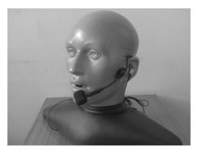
Fig. 3. G.R.A.S artificial head with mounted microphones.
