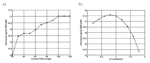
Fig. 4. Output estimate of the speech for the first system as a function of a) control filter order; b) convergence coefficient.
