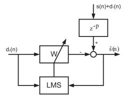
Fig. 1. Feedforward noise compensation.
