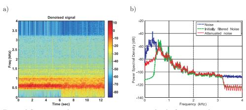
Fig. 6. a) Spectrogram demonstrating noise attenuation for the first system (system starts at the sample 50000), after initial band-pass filtering; b) Noise attenuation for the first system in the frequency domain.
